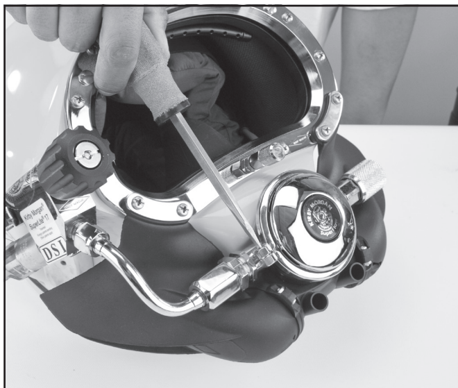
Remove the demand regulator clamp.
