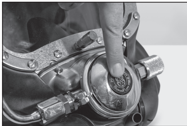
Test the response of the purge button.
