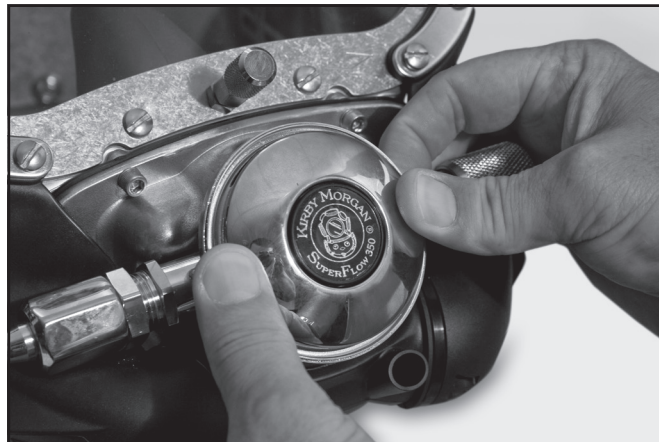
Press the cover over the diaphragm.
