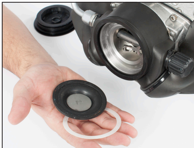
Remove the diaphragm and washer.
