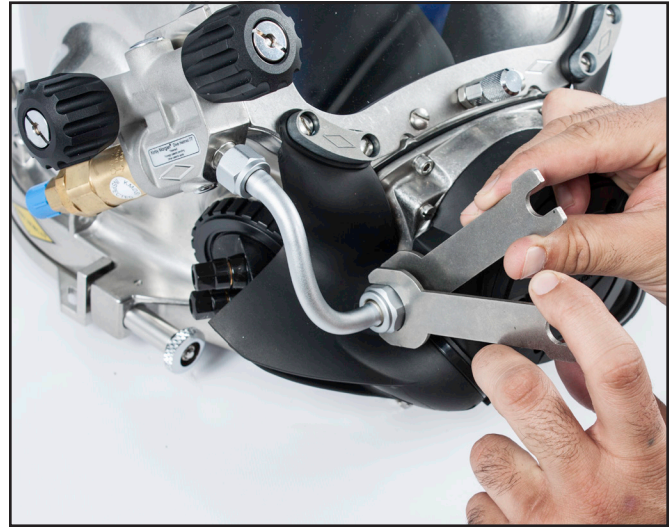
The regulator can be adjusted when it is on the helmet.
