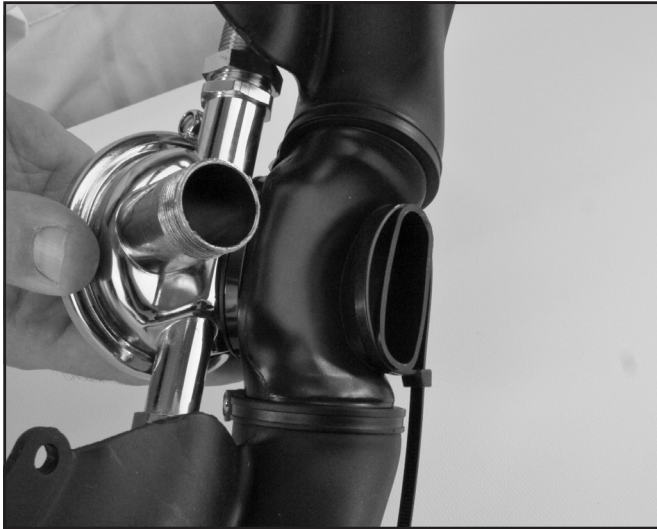
Pre-install the tie wrap.
