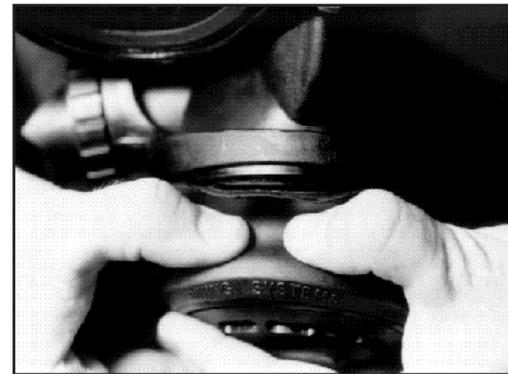
*Incorrect, the whisker is not properly seated. The lip of the whisker seal has come out of the frame.*
