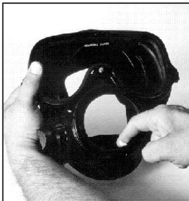
*Lightly grease the regulator opening on the mask seal*
