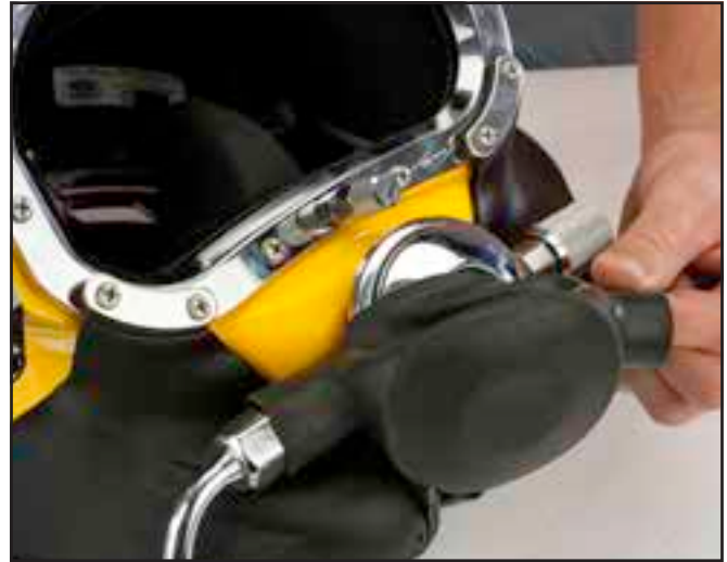
Pull the shroud over the regulator.
