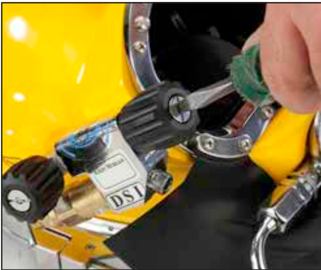
Remove the steady flow knob.
