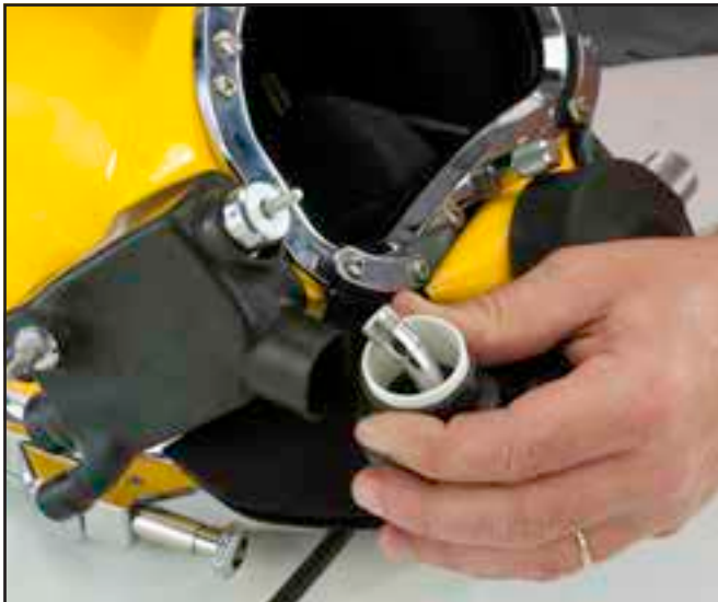
Install the corrugated tube.
