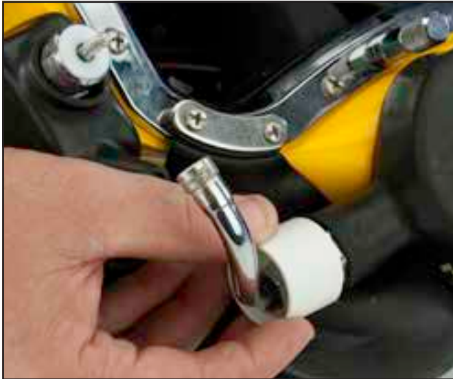
Slide one of the PVC pieces over the bent tube and insert it into the regulator shroud.
