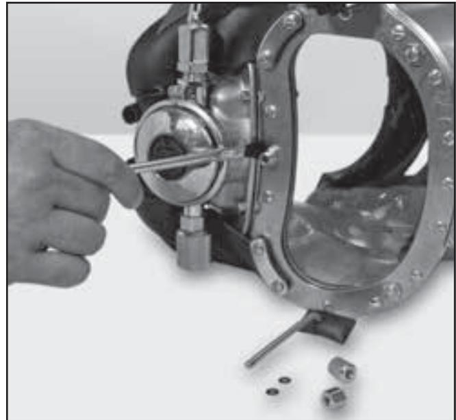
*The threads of the nose block penetrator should be lubricated periodically. All of the parts of the nose block device (with the exception of the O-ring that seals on the back side of the port retainer) can be seen here.*
