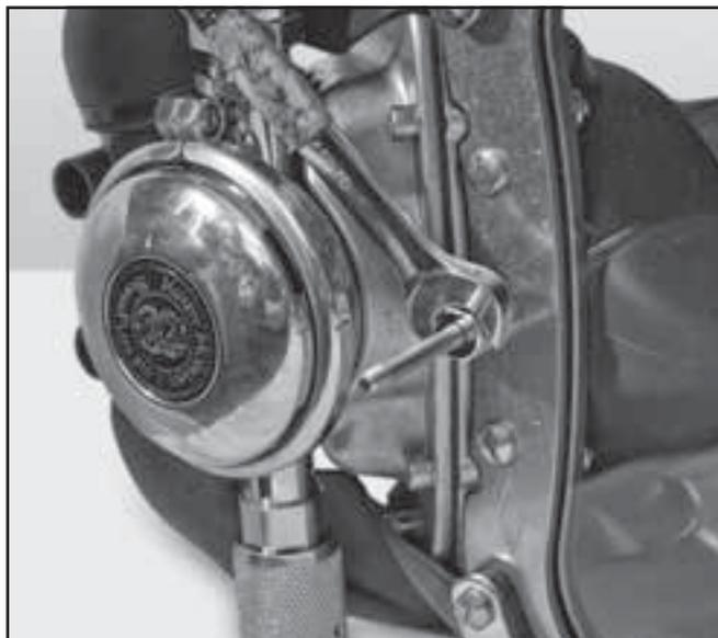
*Do not tighten the nose block packing too much or the nose block device will not slide easily.*
