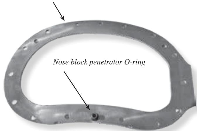
*Be sure to install the O-ring on the back of the port retainer.*
