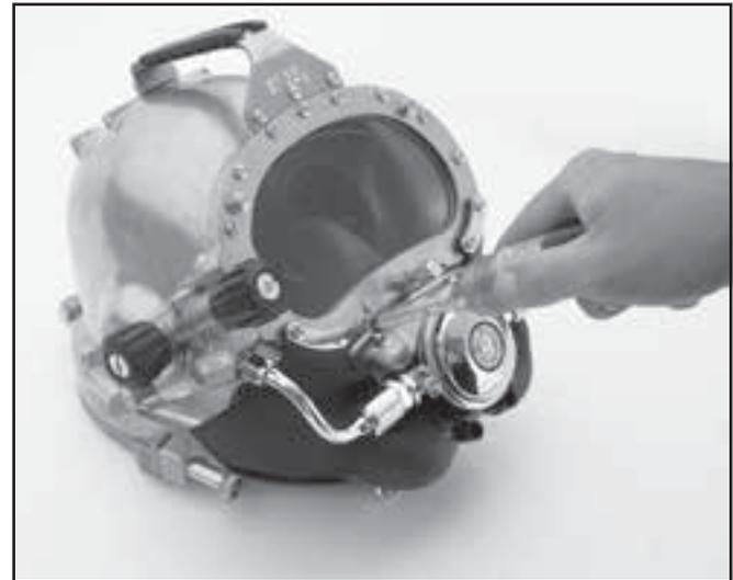
*Remove the screws that secure the port retainer.*
