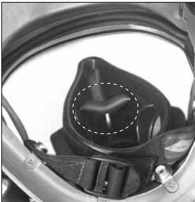
*Properly installed nose block device.*
