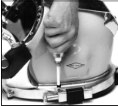
Fig. 6.10 - Remove the screws that hold the sealed pull pins.
