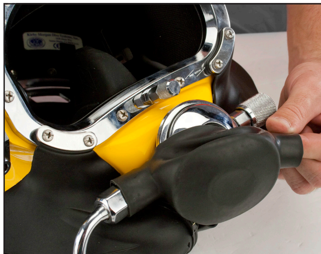
Pull the shroud over the regulator.
