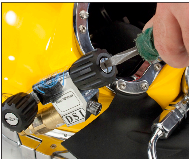
Remove the steady flow knob.
