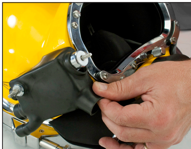
Position the shroud over the side block.
