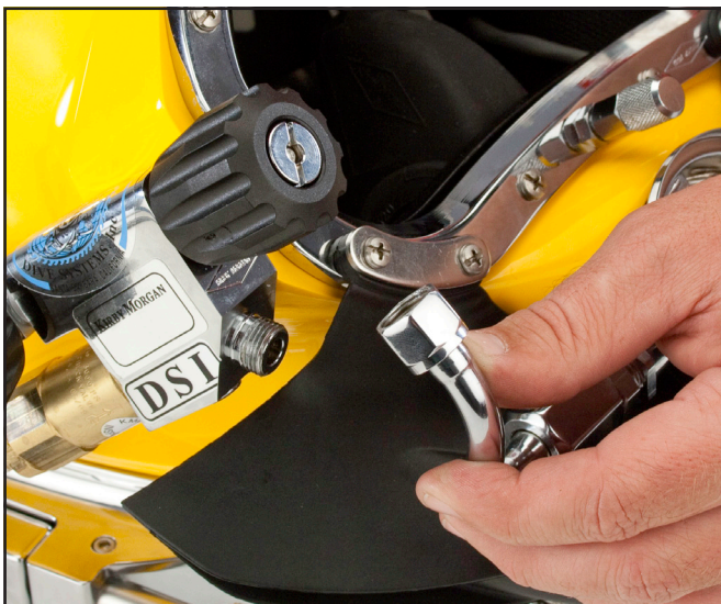
Loosen the bent tube.
