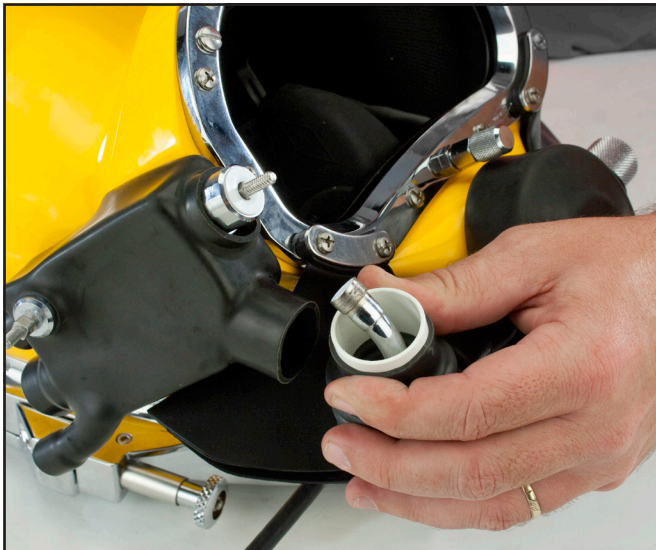
Install the corrugated tube.
