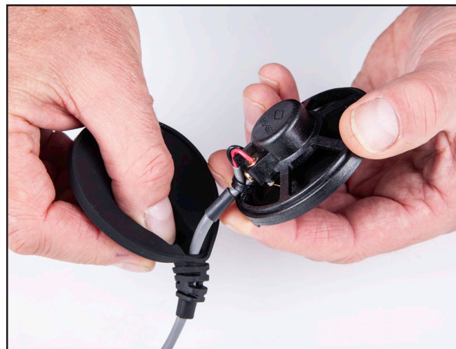
Inspect the mylar earphone.
