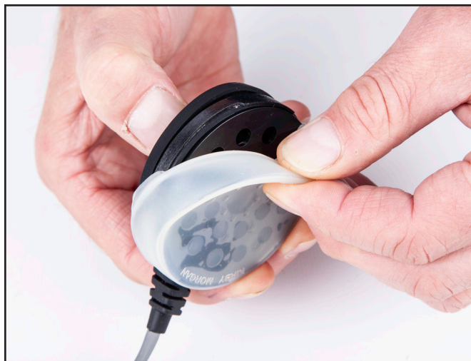
Removing the rubber cover from the earphone.
