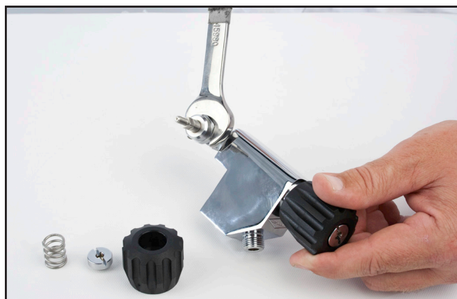
Undo the packing nut.
