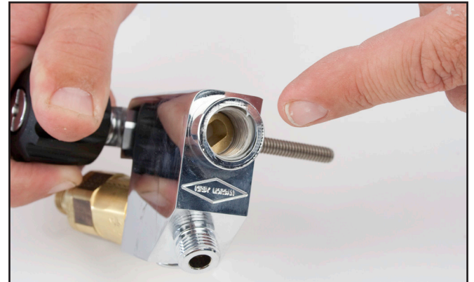
The seat should be removed for inspection.
