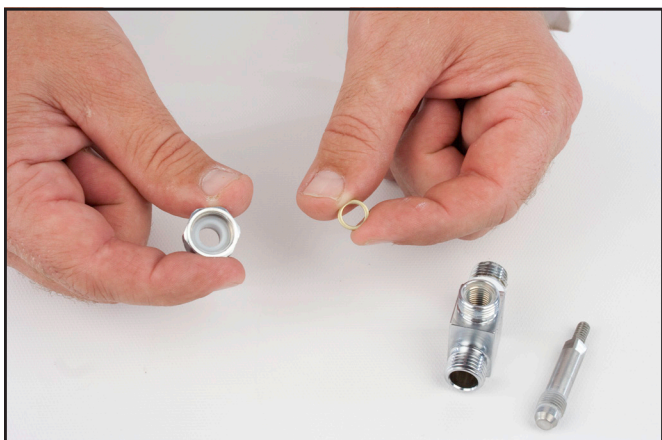
Inspect the packing and washer.
