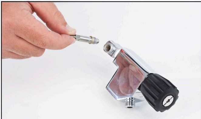
Remove the valve stem.
