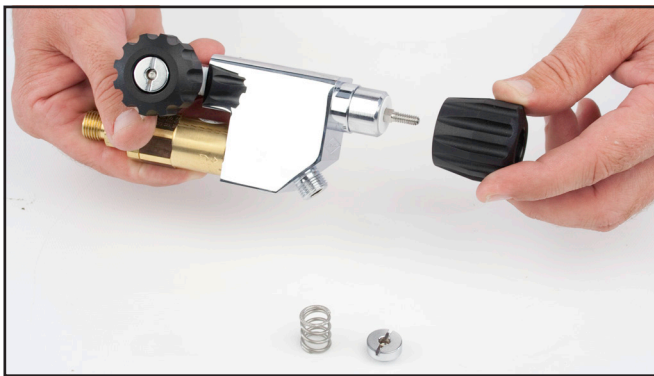
Remove the defogger control knob.
