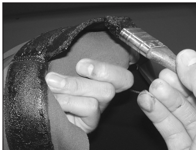
Pre-coat the ear pockets and edges of the ear pocket flap.
