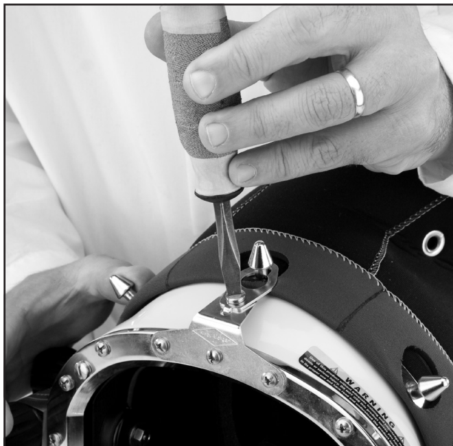
Tightening the top band keeper.
