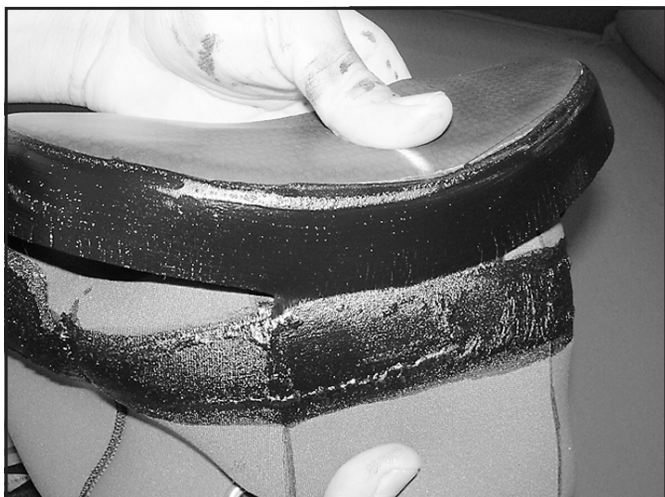
Aligning the top center of the face seal.
