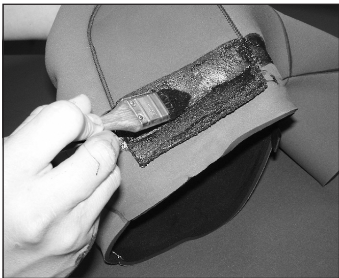
Apply glue to the inside of the hood.
