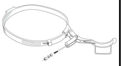
During the clamping process (onto the helmet) one of the welded pins on the neck clamp assembly broke off. On closer inspection it was noted that there was no way of identifying this potential break as both sides of the pin are welded.
