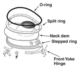
The front yoke hinge on the SuperLite-17C must be the latest version to work with the new stepped ring.
