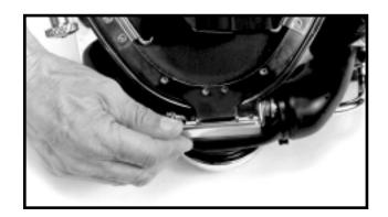
1) Starting January of 1996, the SL-27 and 17C will ship with a new swing catch in place of the tongue catch. This catch allows the diver quicker, easier removal of the helmet. For retrofit upgrades for the SL-27 order part # 525-106,
