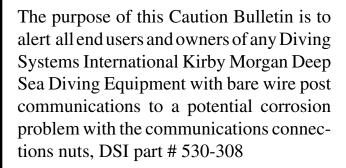
A number of gold plated ferrous metal nuts have recently been shipped in place of our standard gold plated brass nuts. These nuts will corrode in time, especially in heavy salt water use.
