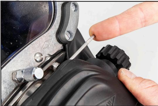
19) Align the access cover, P/N 510-733, to the regulator shroud P/N 510-723, as shown and install the pin, P/N 550-644, until it is evenly located into the area of the regulator shroud where it will remain.
