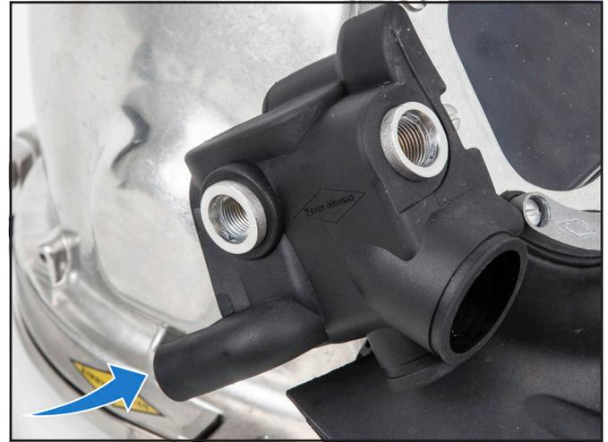
8) Reinstall all of the side block parts that were removed except the bent tube assembly.
