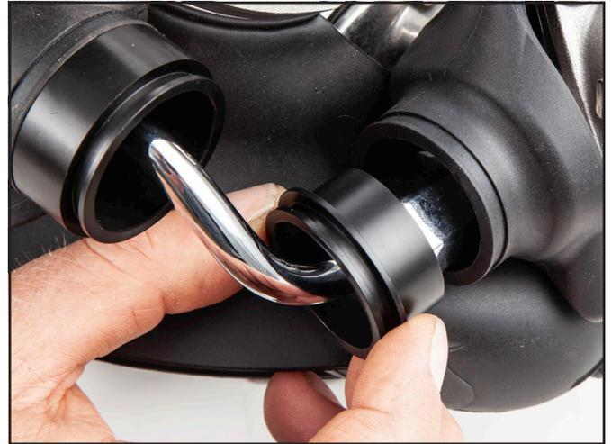
16) Line up the detail features of water tubes A & B, with the mating details of both adapter sleeves.
