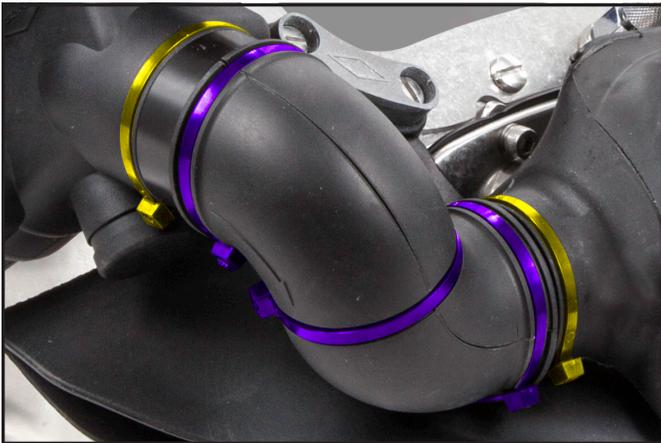
17) Use the three wider tie wraps P/N 520-039 (represented by the purple color in the photo) to secure the two tubes together, one in the middle and one on each of the leading edges of the tube. Little to no gap should be evident between the two tubes.
