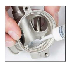
2. Lubricate the internal area of the regulator with approved lubricant where the Main Tube O-ring will insert. This is important to help prevent this O-ring from possibly getting cut when it is installed.
