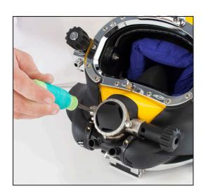
3. Remove the Screws and Washers on either side of the Regulator Cover and unscrew the Cover Retaining Ring.
