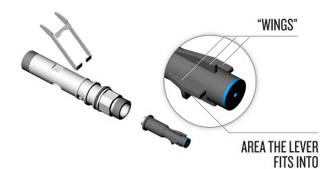
2. Insert the Balance Spacer with the two O-rings installed. Insert the first O-ring into the open end of the inlet valve stainless steel tube and stop at the second O-ring. Next, align and insert the Inlet Valve into the Main Tube, as noted above. If this is done properly, the lever should lift up. If it does not, the Inlet Valve has not been aligned correctly.
