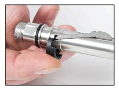
6. Install the Bearing Clip onto the outside of the Main Tube. Note that there is a locating pin on the clip that must engage the correct hole on the Main Tube. There are also small recesses on either side that the legs of the Lever Arm fit into. The clip is correctly positioned when it is in the position shown.
