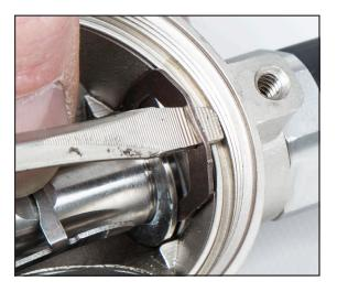
6. Using the 1" open end wrench, loosen the Packing Nut about one turn. Next, while fully depressing the Lever Arm, grasp the Flex Knob and pull it straight out from the Regulator Body. This will remove all of the main components of the regulator valve mechanism as a single, easy to handle unit.
