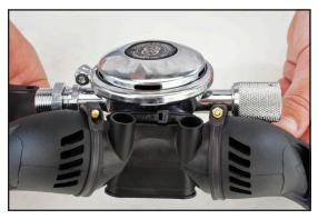
2) Place the tie wrap P/N 520-042 around the tie wrap seating surface on the exhaust assembly and tighten. Make sure that the tie wrap end is positioned as shown. Cut off the excess tie wrap tail.
