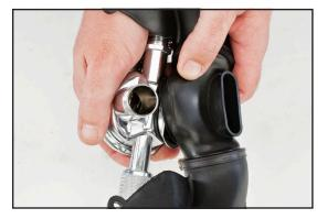
1) Install the Tri-Valve Assembly P/N 505-725 to the regulator exhaust flange.
