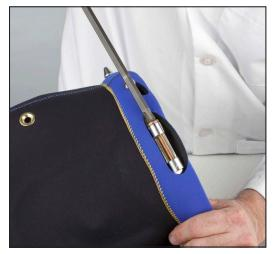
2. Use the bronze band adjustment screws, included in this kit, and start the screws a few threads—just enough to hold the bands together.
