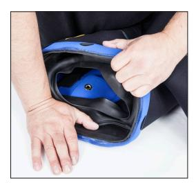
6. Use the palm of your hand or a roller against a table top and carefully work your way around the inside of the face seal and toward the neoprene hood.
