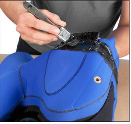
2. Apply the first coat of adhesive to the old adhesive line left behind on the hood from the old face seal.
