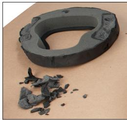
3. Peel off the face seal all the way around the hood. Remove any excess of material left behind, especially the foam on the ear pockets.
