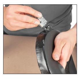
1. Apply the first coat of adhesive to the edge of the new face seal P/N 510-505.
