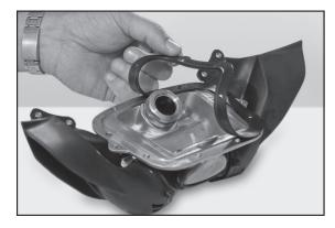
2. Install the gasket. Note the ridge on the gasket. This ridge is designed to help maintain the proper position of the gasket in the groove in the pod.
