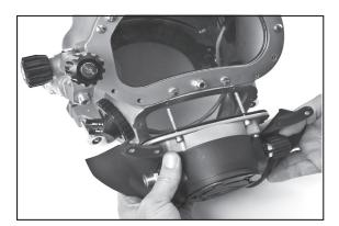
1. See the Stainless Steel Helmets with REX Pod module in your manual for pod removal, remove the pod/regulator assembly from the helmet shell. Remove the nose block device and oral nasal mask, then remove and reserve the oral nasal valve body and valve to be used with the new oral nasal mask.
