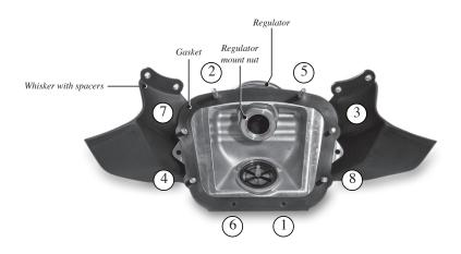
4. Using the 3/2" hex key and 3/8" wrench, tighten the screws onto the helmet. The numbers indicate the order in which the screws and nuts that retain the pod are tightened to connect the pod to the helmet. Tighten the screws gradually, moving from one to another. Do not over**tighten.** Carefully watch the gasket as you tighten the screws—tightening until the gasket barely begins to extrude from between the pod and helmet shell.
