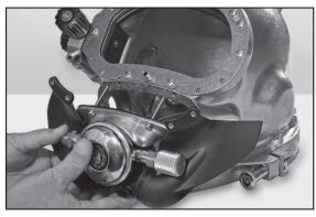
3. Install the new pod/regulator assembly onto the helmet shell.
