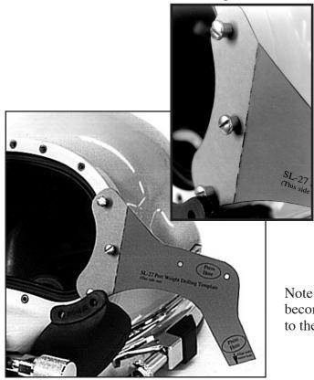
2. Using the whisker spacers on the port retainer screws, secure the drilling template in place on the port side, tightening the screws just enough to hold the template. Bend the drilling template around and onto the port side of the helmet.
