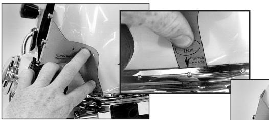
3. Make sure that bottom edge of the template is aligned with the top of the helmet ring, then take a felt tip marker and mark the location of the weight mounting holes.
