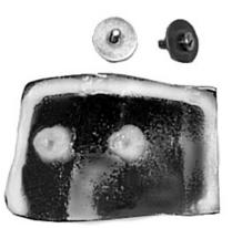
the screw holes as shown. Secure the weight to the helmet using the screws and washers provided. Clean off the excess silicone at this time.
