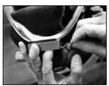
5. Hook spring P/N 535-827 into notch in swing catch and place in position on end of swing catch.
