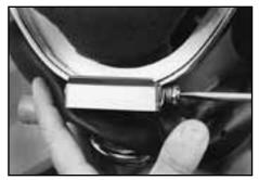
7. Finish tightening screws. Swing catch should close freely and securely with spring pressure.
