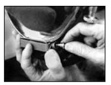
6. Insert spring spacer P/N 550-122 and longer screw through spring, swing catch and Teflon spacer, and start screw into thread in the neck ring. Insure free operation of the swing catch before tightening screws.
