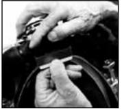
3. Place swing catch in position on neck ring. Bent edge of catch should face in.
