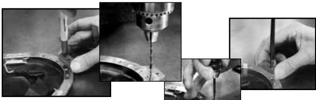
8. Place the neck ring bottom side up and align the small black Delrin tongue spacer on the neck ring tongue. Accurately mark the two holes in the spacer on the neck ring tongue.
