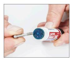
4. If the original screws are being re-used ensure threads are clean and apply a small amount of Loctite<sup>®</sup> 248 onto the ends of the screws. If new screws are used, applying Loctite<sup>®</sup> or other thread locker is not necessary because the screws come with a locking compound already applied.
