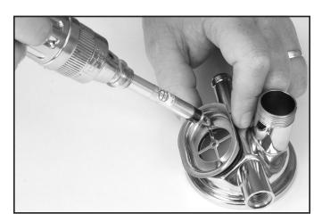
4) Place the screws into the exhaust flange and tighten to 8 inch pounds (0.9 newton meters) and let sit for five minutes then torque to 10 inch pounds (1.13 newton meters).
