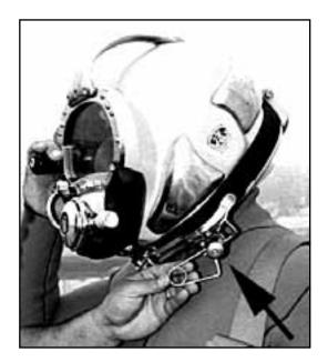
Plunger shaft hole where pin is inserted
