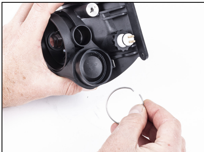
2. Remove the Valve Insert with valve.
