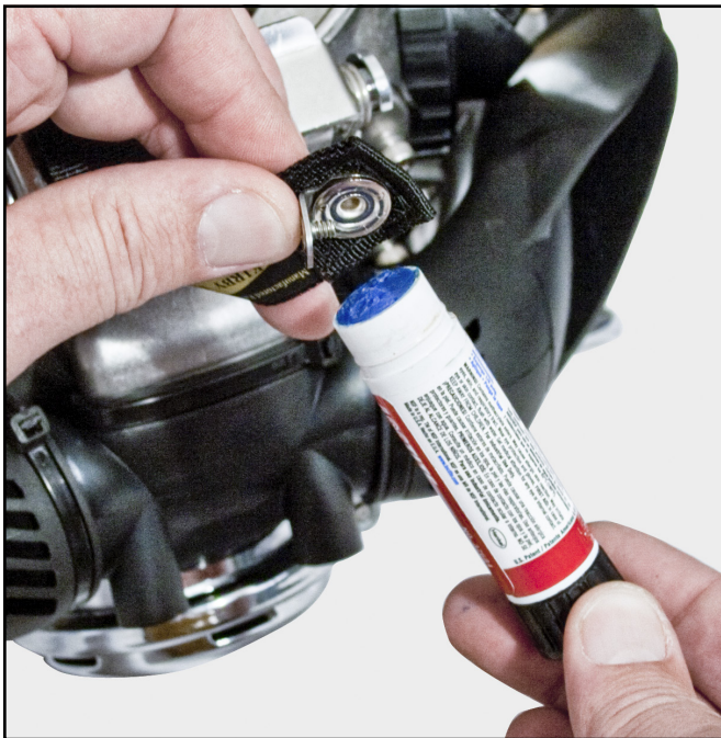
Apply Loctite® to the screws that secure the chin strap.
