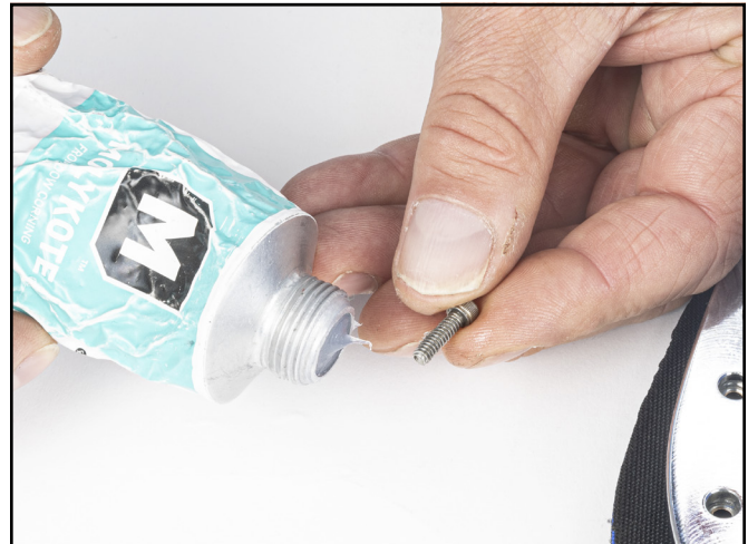
Apply silicone grease to screw tips to ensure smooth installation into the neoprene neck dam.
