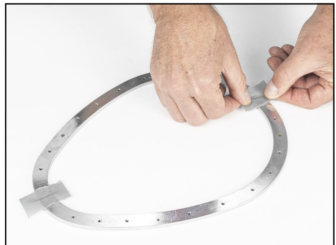
Tape the two rings together with a small bit of duct tape.
