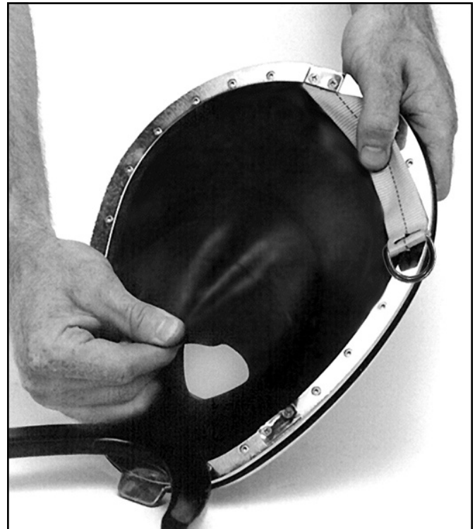
Check the neck dam for holes.
