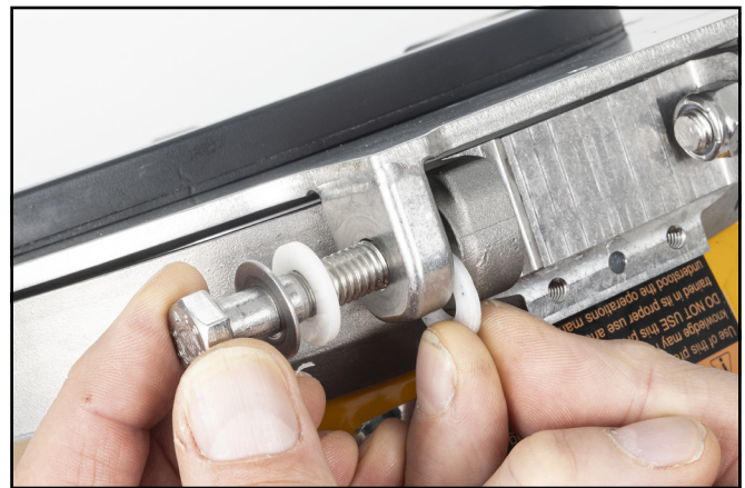
Slide the bolt(s) out from the hinge, taking care not to lose the hard plastic washers.
