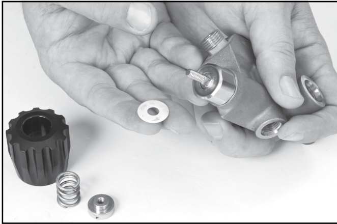
Do not lose the washer that sits between the steady flow valve knob and the bonnet.
