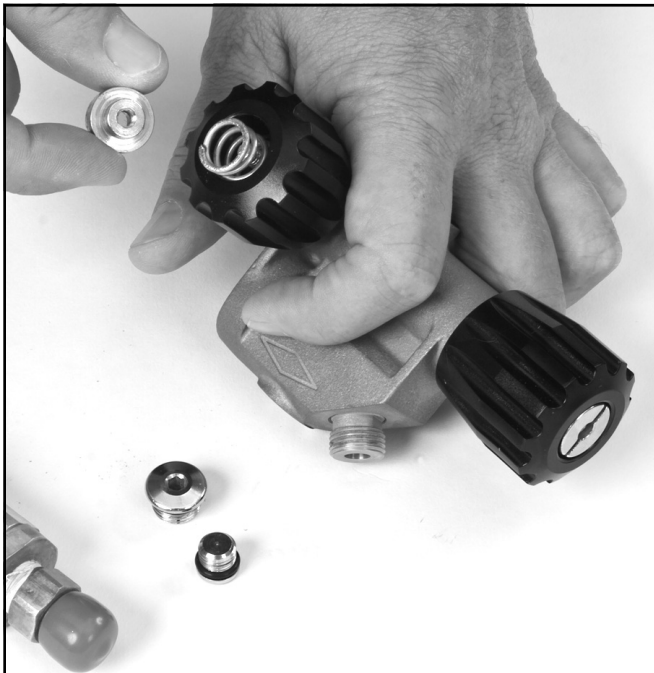
Remove the lock nut and spring
