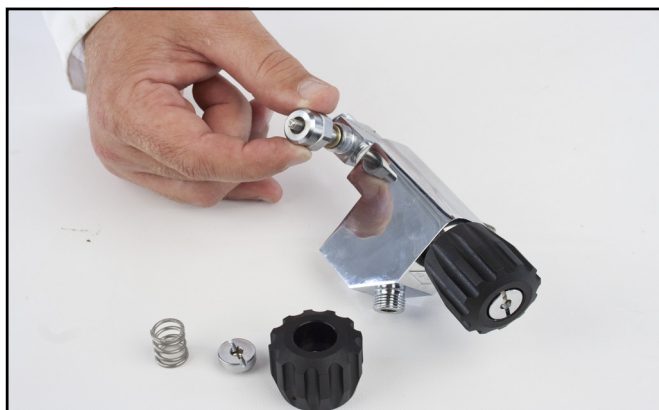
Installing the valve stem into the emergency valve.
