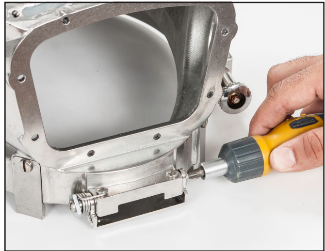
Remove the screw from the port side of the swing catch.
