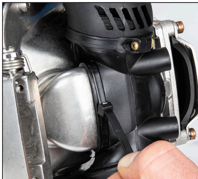
Secure and seal with a tie wrap.
