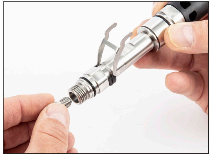
Thread the adjustment nipple into the main tube.
