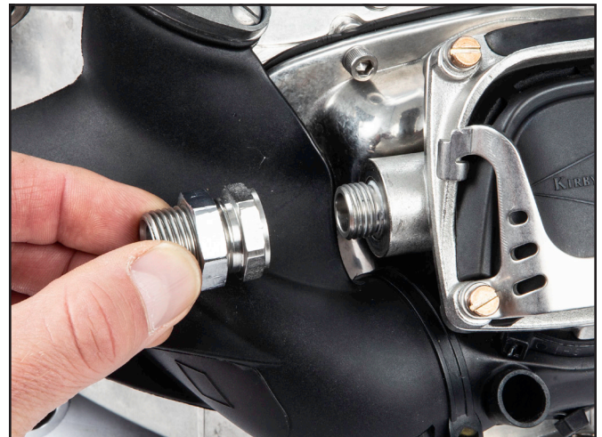
Remove the bent tube adapter.
