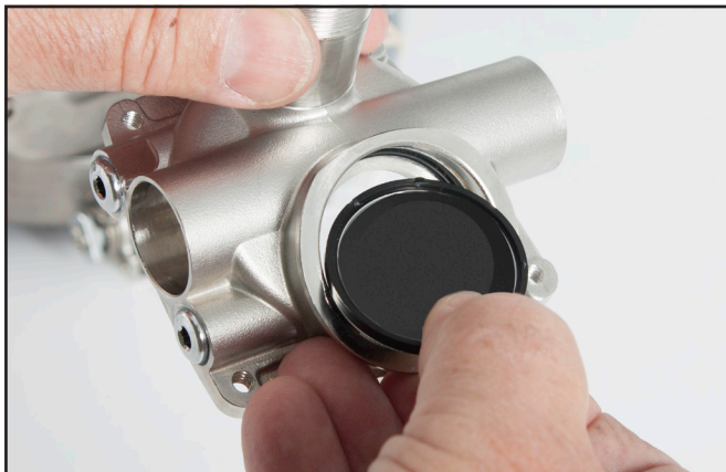
Install the O-ring and valve insert.
