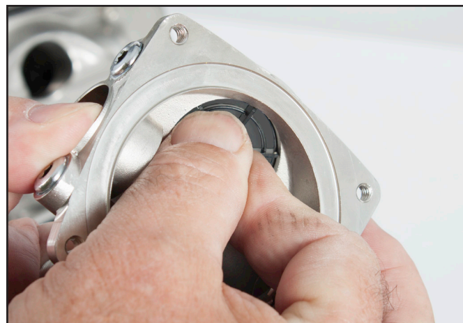
To test to see if the insert is installed properly, try to spin the insert. It should be difficult, or not able to turn.
