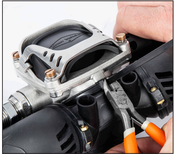
Remove excess tie wrap.
