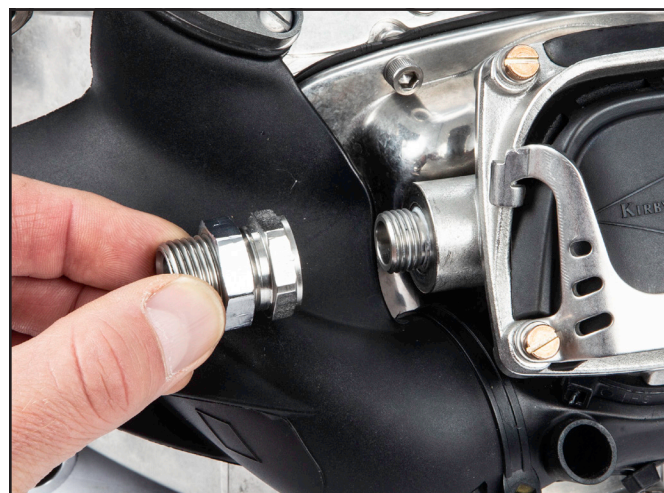
Remove the bent tube adapter.
