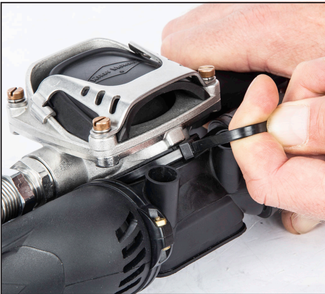
Install the tie wrap on the regulator.
