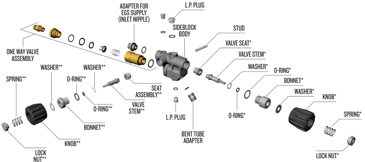
\*\* Components Of Emergency Valve (EGS Valve)
