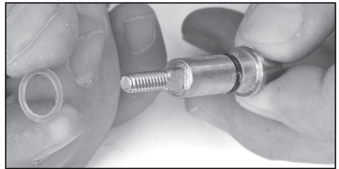
Install the washer on the defogger valve stem.
