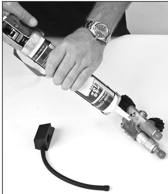
*A small amount of silicone sealant must be evenly applied to the side block prior to installation on the helmet shell. Use only Dow Corning® RTV 732 Multi Purpose sealant or equivalent.*
