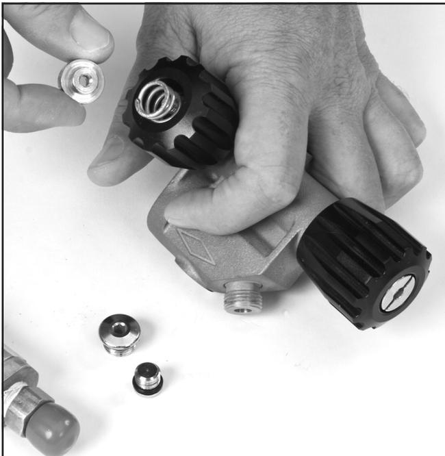
*Remove the lock nut and spring*
