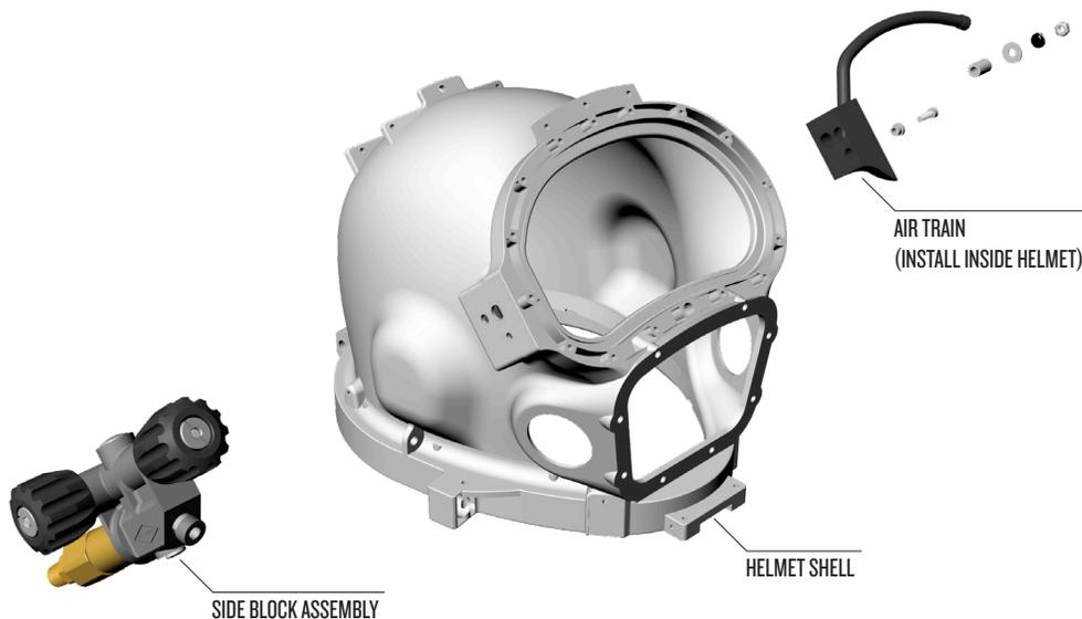
The fasteners that secure the side block also hold the air train in place.
