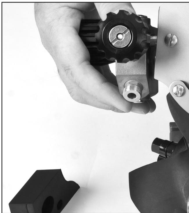
*Install the side block on the helmet shell.*
