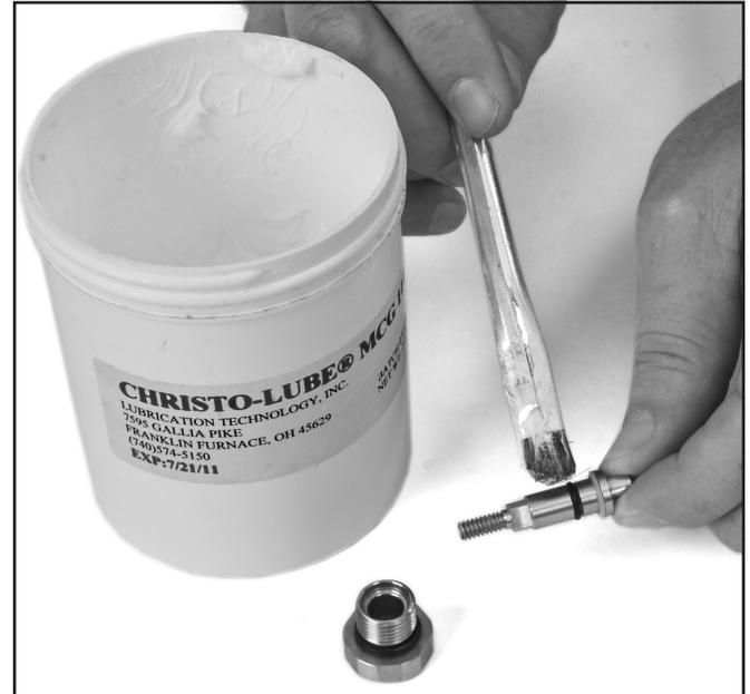
All internal moving parts (with the exception of the valve seat) and O-rings should be regularly lubricated.
