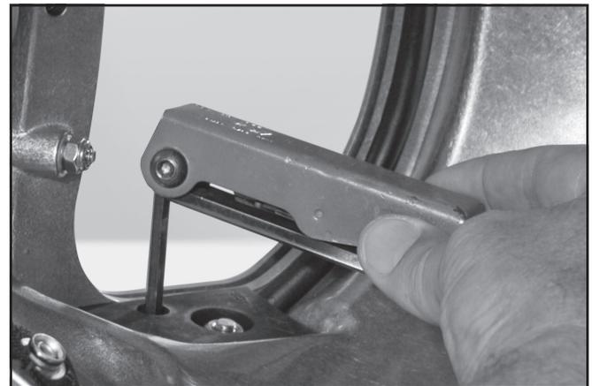
*Remove the alignment stud from within the air train body.*
