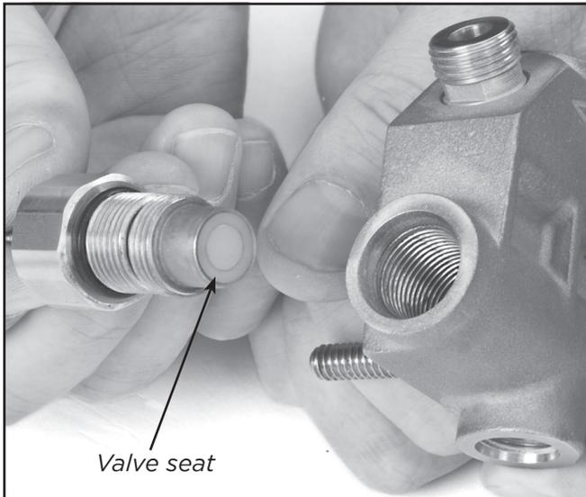
As you unscrew the bonnet, the valve stem and seat will usually come out of the side block together. Note the condition of the seat as shown here. The seat in the defogger valve is a different size than the EGS valve seat. Since the parts have a similar appearance, it is a good idea to keep the parts for the defogger and EGS valve separate. To help prevent incorrect installation and or confusion.
