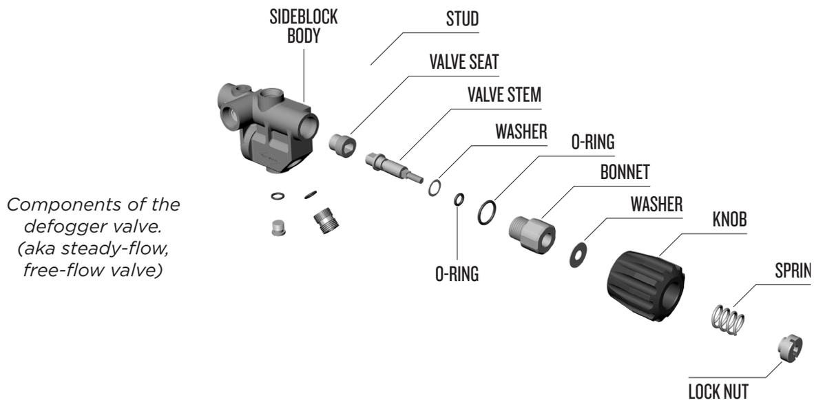
Components of the defogger valve. (aka steady-flow, free-flow valve)
