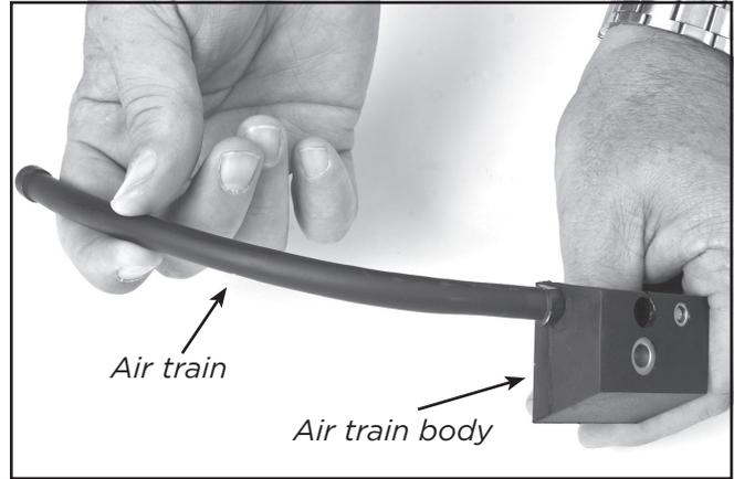
The air train and the air train body are shown above. The air train snaps into the body and is held in place by a small barb on the tube that fits into a matching groove in the rubber air train body. The outer curve of the air train tube must be positioned to sit in the area behind the port retainer with the holes in the tube positioned so that flowing gas from the tube will defog the port.
