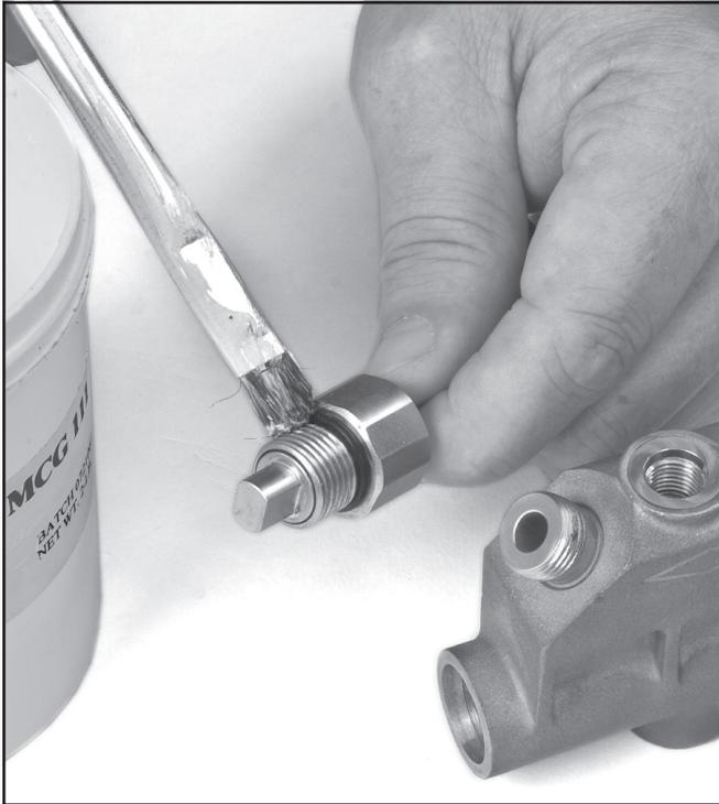
Be sure to lubricate all parts, with the exception of the valve seat, prior to reassembly.
