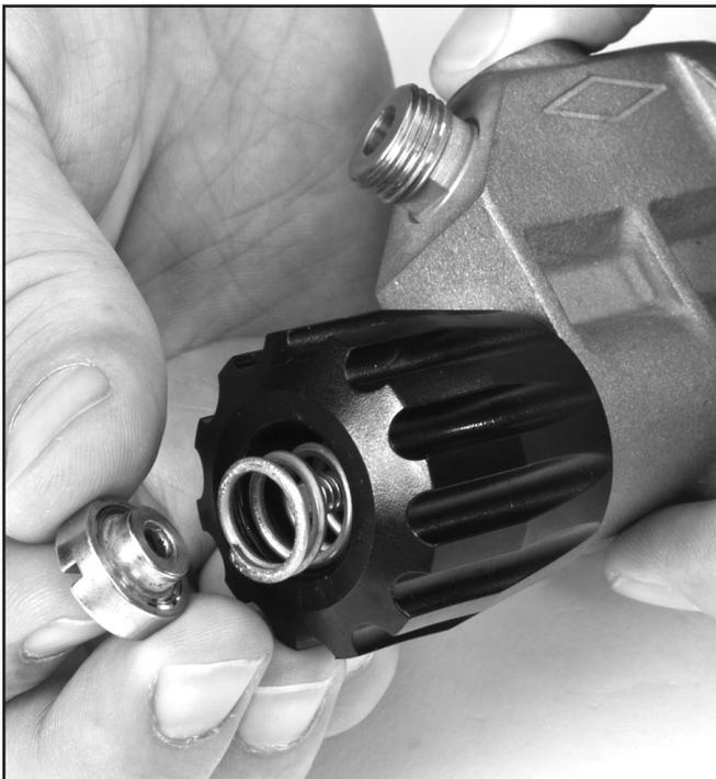
*Remove the nut from the defogger valve knob.*
