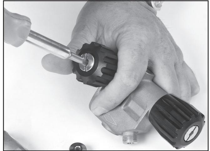
*Tighten the nut that holds the knob in place.*
