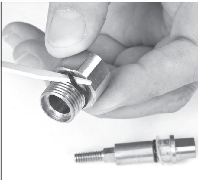
Use a toothpick, credit card, or other non-metal objects to remove the O-rings for cleaning and replacement. Note that the bonnet on the defogger valve is longer than the bonnet on the EGS valve.
