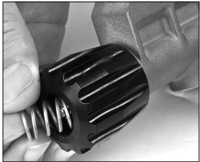
*Install the spring in the defogger valve control knob.*
