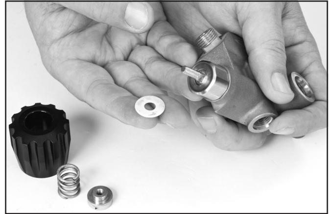
*Do not lose the washer that sits between the defogger valve knob and the bonnet.*
