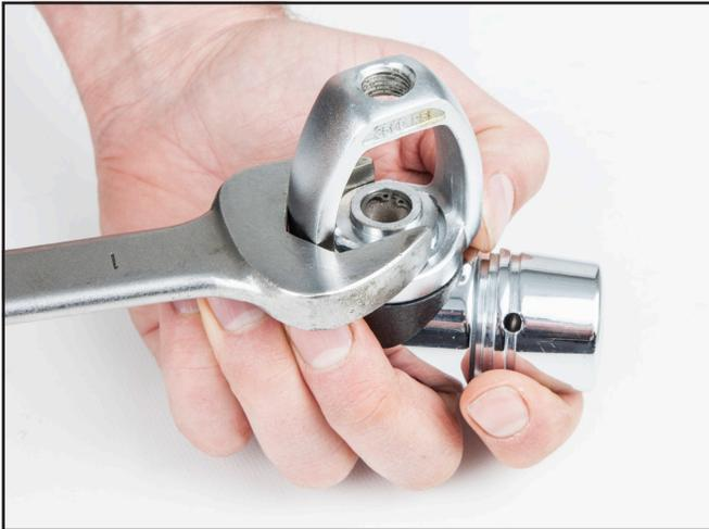
26) Thread the Yoke retainer, saddle and yoke as an assembly into the regulator body.
