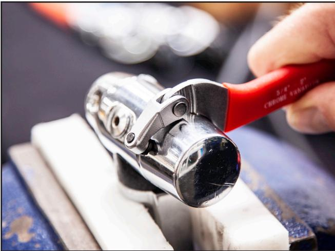
19) Screw the cap in, until the assembly is snug. Tighten with a spanner wrench.
