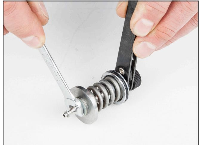
7) Use the 1/4" nut driver to loosen and remove the nut from the opposite end of the poppet.
