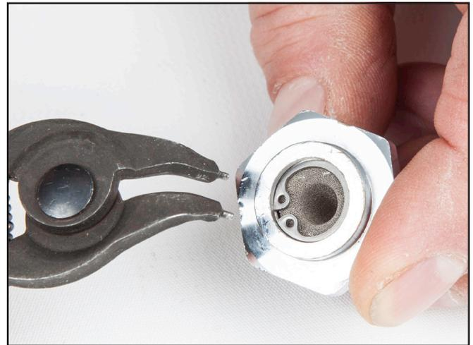
18) Remove and inspect the filter for oxidation and contamination. If the filter is corroded or shows visual signs of contamination it must be replaced. When in doubt, replace the filter.
