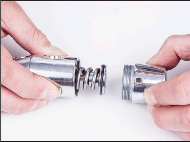
18) Place the first stage body in a padded vise. Tighten the vise just enough to hold the regulator body.
