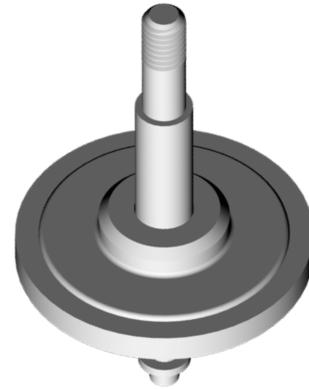
7) If shims were present in the regulator, install the shims in the recessed groove in the piston head.
