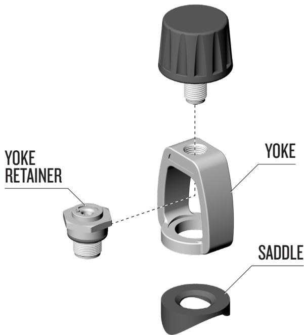
16) Remove two O-rings from the yoke retainer.
