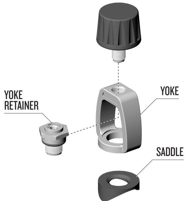
24) Install the saddle on the yoke retainer.
