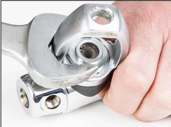
13) Unscrew the yoke assembly from the regulator body.
