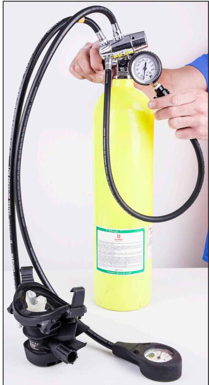
2) If the pressure creeps more than 10 psig (0.7 bar) within 5 minutes, it is an indication that the poppet and seat are not sealing properly. Depressurize the system, then repressurize and check for intermediate pressure creep. If the regulator continues to creep, the poppet and/or seat may be
