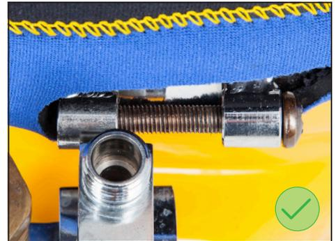
Make certain the bands are over the rubber of the molded face seal and the neoprene has NOT folded over the rubber.
