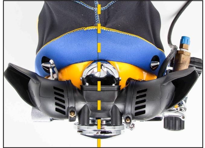
5. Using a torque screwdriver with a large Phillips attachment, torque the band screws to 26 inch pounds\* (2.94 Newton Meters).
