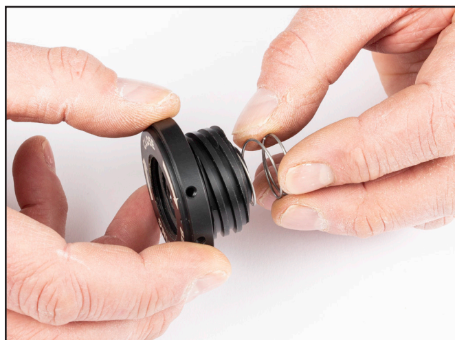
9. Turn Spring clockwise and slightly apply pull pressure to separate from body.
