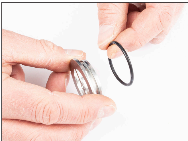
13. Remove Housing Retainer Ring.
