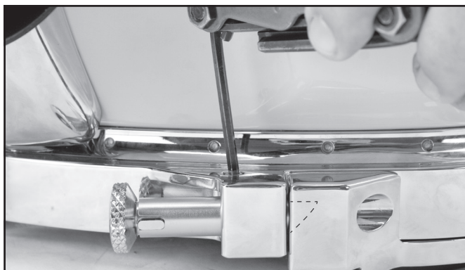
Unscrew the hex head screws
