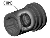
3. Apply a liberal amount of Christo-Lube or equivalent non-silicone lubricant to the threads of the slot shaft.
