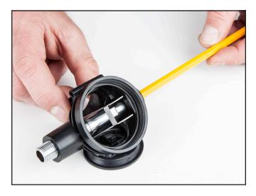
The lever arm should rise up toward diaphragm area with this increasing pressure.
