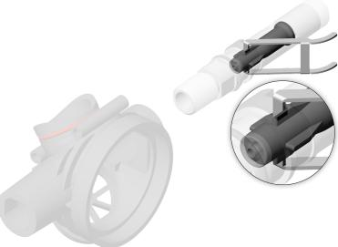
7. With the main tube still positioned in the center of the regulator body, use the eraser side of a pencil to gently and steadily push onto the inlet valve from the adjustment knob side of the main tube.
