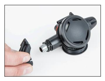
7. Install exhaust whisker firmly in place, making sure orientation of outlet ports is correct, as shown.
