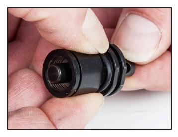
13. Turn the slot shaft into packing nut clockwise until free of packing nut.
