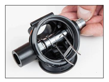
5. Install or inspect soft seat on inlet valve.
