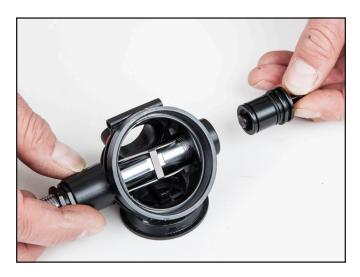
12. Remove the O-ring found on the outside of the packing nut.
