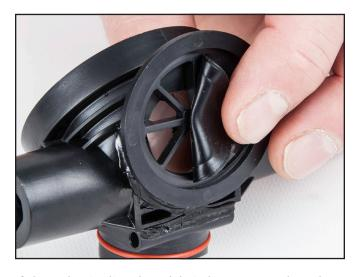
If the valve is discolored, brittle or warped, replace valve.
