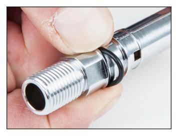
26. Using a flat blade screwdriver, loosen the inlet nipple counter clockwise, enough so that it can be pushed out of the main tube using a wooden dowel, chop stick or sharpened end of a pencil. These items will prevent damage to the sealing edge of the nipple.
