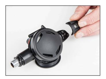
5. Install adjustment knob screw and tighten until snug. There should be no gap between knob halves.
