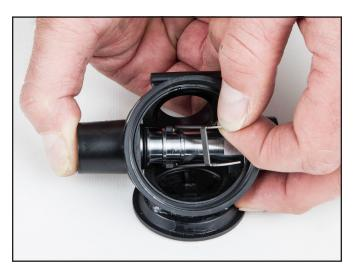
This causes lever arm to slide away from interior wall of regulator body, allowing for its removal.
