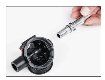
24. Note position of bearing clip as reference for correct reinstallation. Remove bearing clip from main tube.
