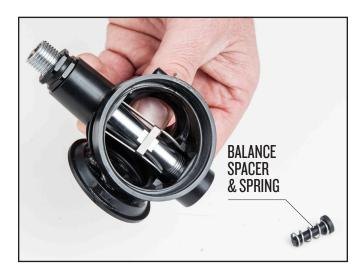
16. Remove O-ring on balance spacer. (Discard if performing a yearly overhaul)
