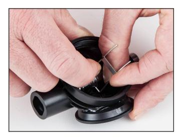
20. Pull second leg out and free from hole, then remove entire lever arm from the main tube.
