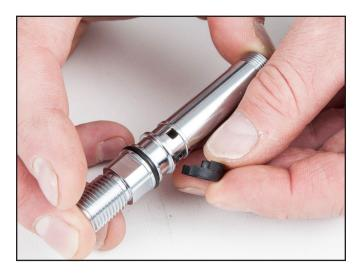
25. Remove O-ring from main tube (discard if performing a complete overhaul).
