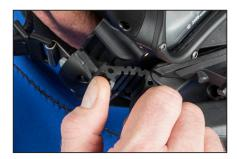
Squeeze the front and the back parts of the pod Catch, Release together to release the pod from the mask. Swing the pod forward and to the left in an arcing motion to free the pod Hook from the mask.
