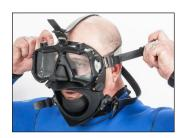
3. Pushing the mask up onto your face, get your chin and the nose dam positioned comfortably into the mask, then lightly tighten the Temple Straps first only enough to position the larger area (junction) of the harness at the back of the head and as low as possible.
