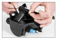
8. Using tie wrap tool or equivalent, install new tie wrap to secure Purge Tube in place on pod skirt.
