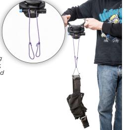
If there is any doubt regarding the mounting of the regulator, perform a pull test as illustrated here, by using a 25 lb. weight.
