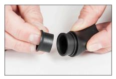
6. Insert purge sleeve into purge tube, as shown. Make certain the direction of the sleeve is correct and that it is pushed all the way into the purge tube.
