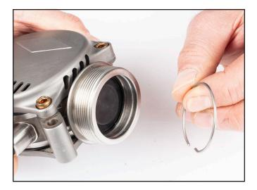
6) Lubricate O-ring and install onto Puck Seal.
