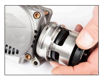
13) Place Split Retainer onto control Control Knob, aligning the holes.
