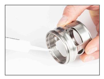
4) Thread Exhaust Control body with Spring into Retainer Housing.
