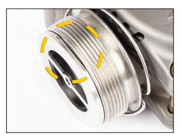
11) Use large flat blade screwdriver and **remove** with an even pull outward.
