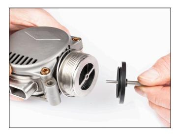
7) Orientate exhaust assembly so stem is pointing up and exhaust body, as shown.
