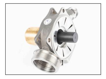
4) Once tools are secured use  $\frac{3}{4}$ " wrench to turn large bronze handle clockwise to loosen.
