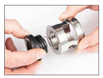
9) Turn Spring clockwise and slightly apply pull pressure to separate from body.
