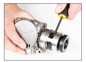
11) Secure housing Retainer Ring onto Retainer Housing, one hook end at a time, using your fingers to work the ring around the housing until the other hook end is secure.
