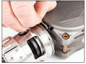
3) Use 3/16" Allen Wrench to rotate counter clockwise the retainer housing.
