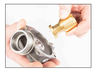
2) Position assembly so the large brass removal tool is down with the slotted Valve Seat facing up.
