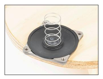
8) Lower regulator body onto the bottom diaphragm cover with diaphragm and spring in place.
