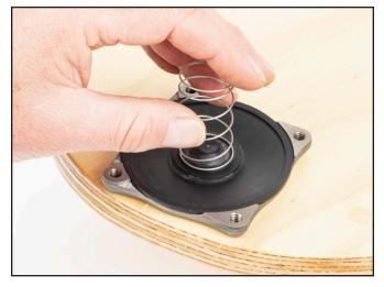
7) Center Diaphragm with Spring onto bottom (screen) cover with even gaps all around the leading edge.
