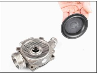
19) Complete disassembly of exhaust regulator– Bottom cover, 2nd Stage Diaphragm and Spring.
