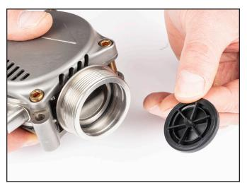
5) Insert Retainer Ring into OPRV body.
