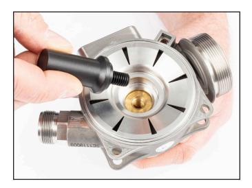
The threaded end of the tool will go through the hole and mate to removal tool that is secured from the screen side (second stage) of the exhaust regulator.
