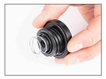
3) Lubricate internal threads found inside Retainer Housing.
