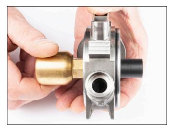
10) Use ¾" wrench to turn large bronze handle counter clockwise to tighten.
