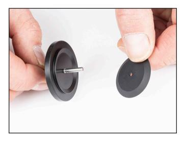
8) Unscrew Exhaust Control Body and separate from housing.
