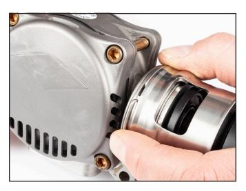
12) Rotate Control Knob out slightly to make room for adjustment knob halves.
