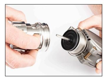
5) Remove Puck with Pin and large spring and set aside.
