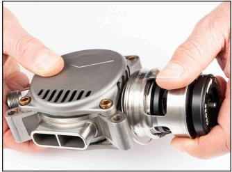
10) Use  $\frac{3}{16}$ " Allen wrench to snug housing onto body.
