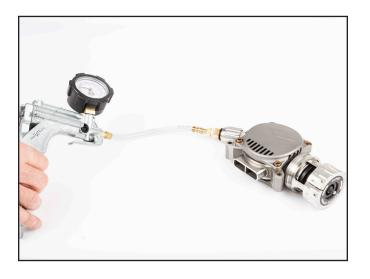
3) Block off mount tube with Hand or flat surface to initiate vacuum lock up.
