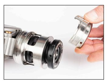
14) Tighten hex screws until the top of the screw is just barely below the outer surface of the knob.
