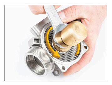
Tighten– TURN Counter clockwise Only tighten until the Valve Seat bottoms out.
