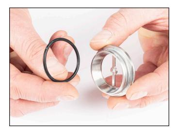
7) Insert evenly into exhaust valve body.
