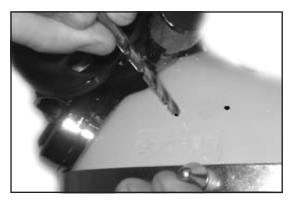
4) To Drill the holes accurately use a Drill Start or twist the Drill Bit by hand to start the holes first to prevent the drill from wandering. Use a #10 (0.1935") Drill and carefully drill the two holes.
