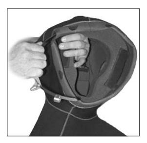
9) Remove the Adjustment Screws from the Bands and feed the Bands into the Hood through one of the large holes on the sides.
