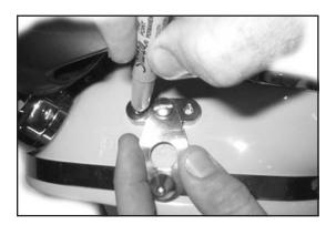
2) Install the Bottom Band Keeper Attachment Plate onto the Bottom Band Keeper Mount using Screw (P/N 530-073) with the bend towards the Mount and so that it creates a "T" like shape. Place this assembly onto the lower port side Head Harness Mount Stud as shown leaving a small ( $\frac{1}{16}$ ") gap between the end of the slot in the Keeper Attachment Plate and the Head Harness Mount Stud. Then use a pen to mark the location of where the mounting holes need to be drilled as shown.
