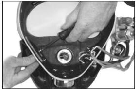
7) Install the Bottom Band Keeper Mount onto the outside of the Mask Frame using two Screws (P/N 530-062) and torque to 14 inch pounds. Clean off excess Silicone.
