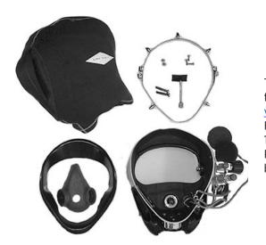
The following parts must be removed from your KMB 18/28. Refer to the KMB 18/28 Manual which can also be found online at <a href="https://www.kirbymorgan.com">www.kirbymorgan.com</a> for removal procedures. Remove the Head Harness (Spider), Hood, Top & Bottom Bands, Comfort Insert (KMB 18's Only) Nose Block Device, Oral Nasal and the Three Top Port Retainer Screws. Inspect and replace if necessary parts that will be reused for the installation of the new Hood & Band Keepers.
