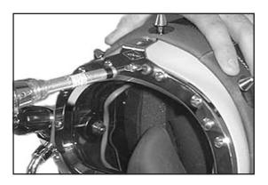
13) Install the Top Band Keeper Mount onto the front of the Port Retainer using three Screws (P/N 530-040) and tighten them with a Torque Screwdriver to 12 inch pounds.
