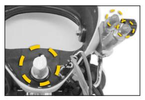
3) Cap or plug the Regulator Mount Tube, One Way Valve Adapter and Emergency Valve Inlet to prevent debris from entering during drilling
