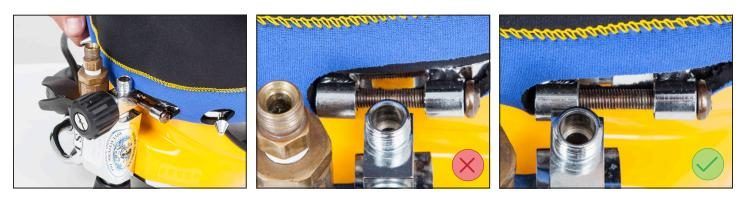
Make certain the bands are over the rubber of the molded face seal and the neoprene has NOT folded over the rubber.
