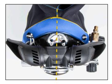
6. Using a torque screwdriver with a large Phillips attachment, torque the band screws to 26 inch pounds\* (2.94 Newton Meters).
