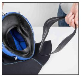
3. Install the face seal spacer P/N 520-153 into the molded face seal. (Only the KMB 28 Band Masks require this spacer. KMB 18s do not).
