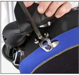
1. Remove the band keepers P/N 540-175 and 540-179.
