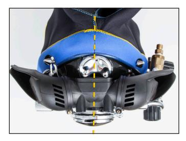
6. Using a torque screwdriver with a large Phillips attachment, torque the band screws to 26 inch pounds\* (2.94 Newton Meters).
