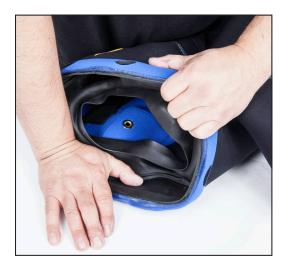
19. Use the palm of your hand or a roller against a table top and carefully work your way around the inside of the face seal and toward the neoprene hood.
