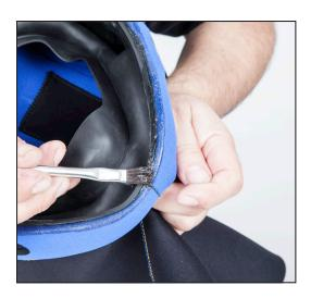
21. Apply a coat of Aquaseal to the front of the hood and face seal combination, along the front edge of the face seal. Spread the Aquaseal evenly, making sure it overlaps, from the edge of the face seal onto the hood by about ½ inch (6.35 mm).
