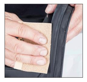
10. Using 120 grit sandpaper, sand a 1 ¼ inch (3.175 cm) wide strip all the way around the outside edge of the face seal. This 1 1/4 inch (3.175 cm) strip will be the mating surface for the neoprene hood
