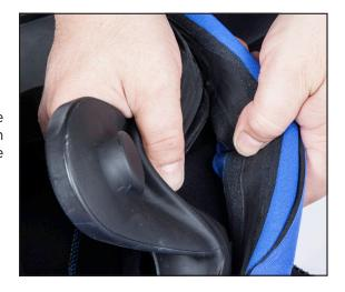
9. Remove any leftover bits and pieces of face seal or Aquaseal\* left behind.
