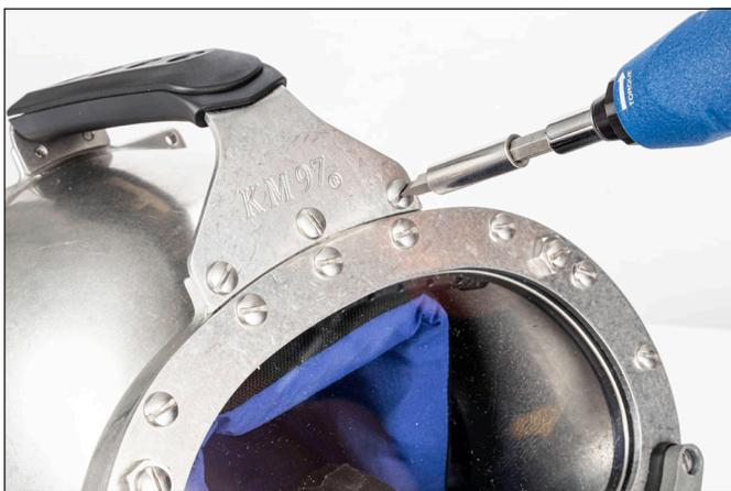
9) Reinstall the handle onto the helmet. Refer to “1.1.3 Handle Replacement On Stainless Steel Helmets” on page SSHNDL-6 of the “Handle on Stainless Steel Helmets” module.
