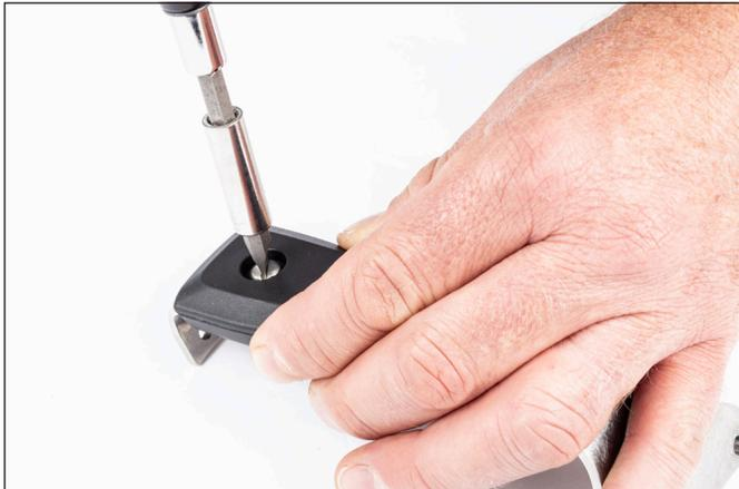
8) Apply Loctite® 248 to the screws and install. Torque to 15 Inch Pounds (1.7 Newton Meters).
