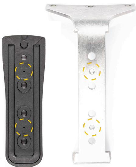
*Underside of the handle top indicating where to drill holes (#7, 0.201”) and corresponding holes on the topside of the handle, in order to use the original grip mounting holes in the handle (10-32 UNF Screw).*
